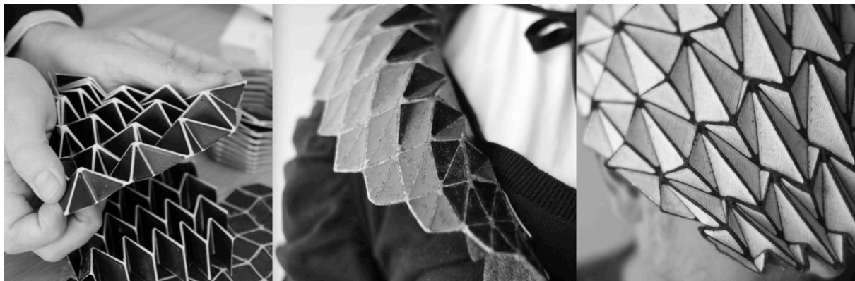
Figure 1. Advanced multi-material prototypes. Left: a set of regular corrugations (waterbomb, miura, and yoshimura). Center: Irregular yoshimura-based fashion prototype in felt, polymer and elastomer. Right: Irregular waterbomb pattern formed into a cap.
